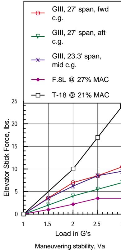
imum G evaluated. The control forces felt light enough for good maneuvering yet had high enough feedback to assure accurate pitch control. ( See graph).
