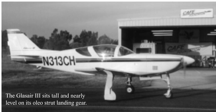
The Glasair III sits tall and nearly level on its oleo strut landing gear.
