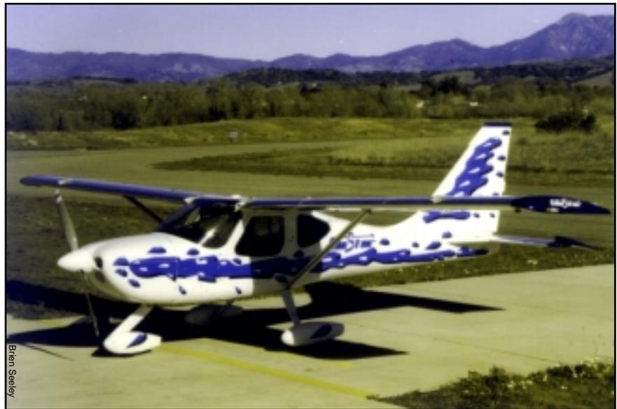
stick was rapidly oscillated out of phase with the control surface movement while seated in the stationary aircraft. (In flight, the aileron's trailing edges were observed to reflex upward about 3/4" relative to their relaxed position on the ground.) These problems could be partly attributable to poor rigging or to the heavy use seen by the prototype, but even several thousand airframe hours should not alter the control system significantly.
