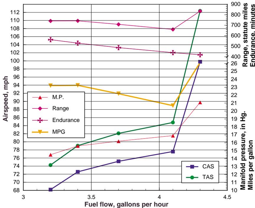
GlaStar N824G: low power settings. All data at 6000' density and 2080 rpm except the 112 mph TAS data point which was at 8000' density and 1800 rpm.
