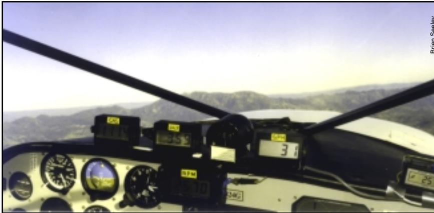
The CAFE flight data is displayed digitally by LCD boxes taped atop the glare shield.
