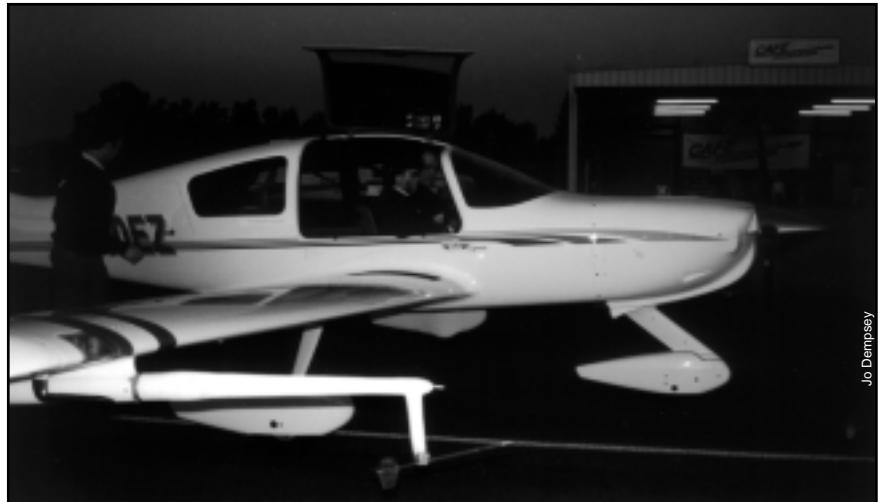
CAFE Barograph, pitot-static and boom mounted on rt. wing for first data flight at dawn on 9/20/97. Note large, gull-wing cabin door and rear baggage door.
