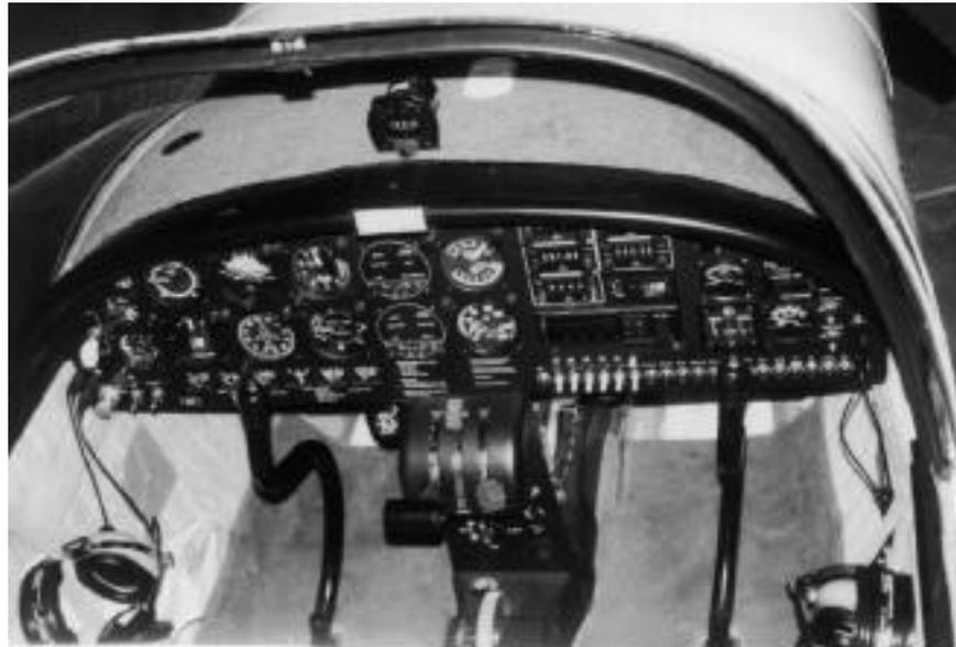
fashion in accordance with the written checklist. Flaps were set to 15 degrees for take off as recommended. A very nice and well marked elevator trim wheel was set to the recommended position. The magnetos checked out OK with the only note being that the panel-mounted analog tachometer read 70-80 RPM below the accurate digital tachometer. A dual function volt/amp meter had been installed and worked well, providing an accurate indication of the condition of the electrical system.
