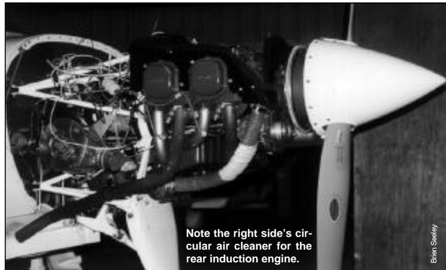
Note the right side's circular air cleaner for the rear induction engine.
