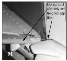
an airfoil-like shape. This can be accomplished by glueing piece of foam onto the aft face of a strut or antenna and then shaping the foam to taper with a 3 or 4 to one fineness ratio. (M)
