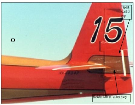
gap flow a significant source of both 'leakage' and interference drag.
