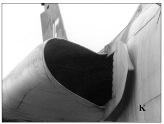
in order to not inhale the boundary layer. The F-105 engine inlets used a boundary layer bleedoff fence that enclosed a flow dividing 'prow'. (**K**).
