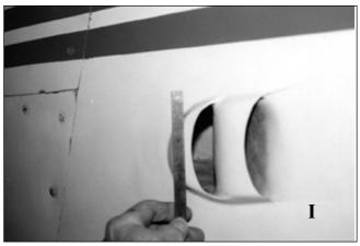
area, the wake and therefore the drag of the bluff body extractor exit can be kept small. The internal walls of the exit should create a convergent path for the air to accelerate it as it exits. The extractor shown in **A**, **C** and **D** incorporates an adjustable cowl flap consisting of an internally-opening, aft-hinged door. The
