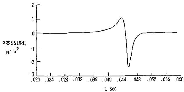
Figure 4(a) Thickness Noise, 45° Azimuth
