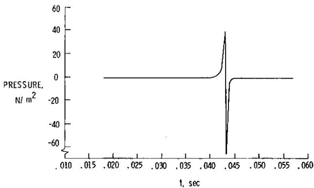
Figure 2(a) Thickness Noise, In-plane
