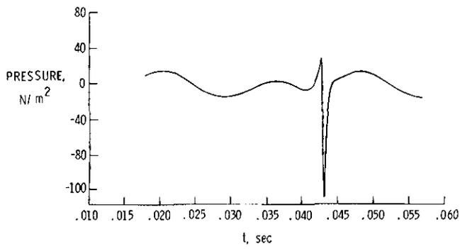
Figure 3(b) Total Noise, In-plane,  $\omega_h = 2\Omega$
