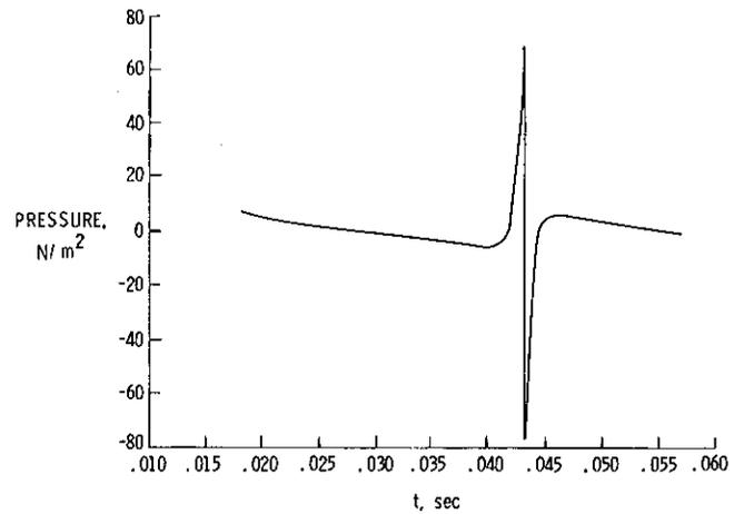
Figure 2(c) Total Noise, 6° Angle of Attack, In-plane
