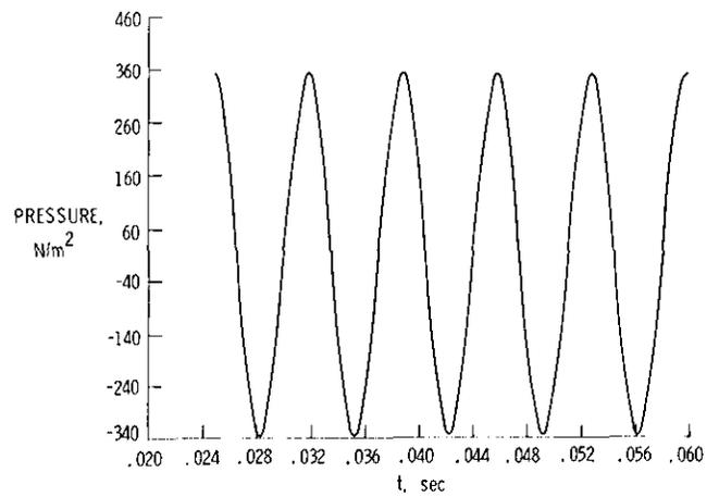
Figure 5 Total Noise, On Propeller Axis,  $\omega_h = 4\Omega$
