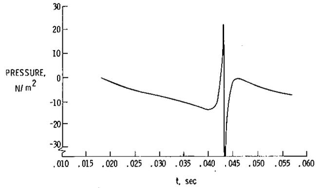
Figure 2(b) Lift Noise, 6° Angle of Attack, In-plane
