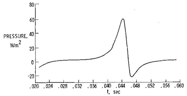
Figure 4(b) Lift Noise, 45° Azimuth
