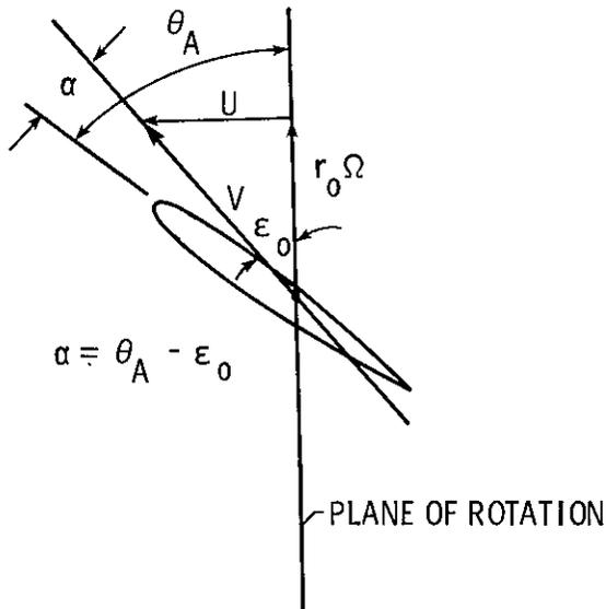
Figure 1(b) Coordinate System - blade cross-section
