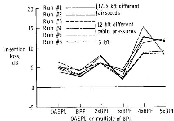
Fig. 7 Space averaged insertion loss for OASPL and multiples of the BPF for six flight conditions.
