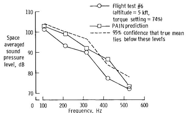
**Fig. 11** Measured and predicted space averaged sound pressure levels (treated airplane, 74% high engine torque).
