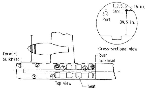
**Fig. 1** Microphone locations relative to the interior plan of the treated airplane.
