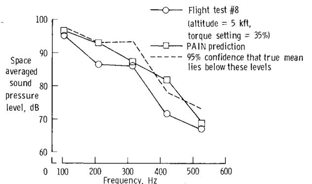
**Fig. 12** Measured and predicted space averaged sound pressure levels (treated airplane, 35% low engine torque).
