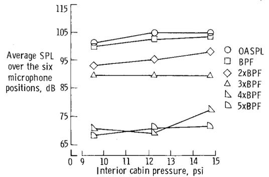
**Fig. 9** Effects of cabin pressure on space averaged sound pressure levels for the treated airplane.
