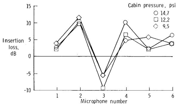
Fig. 5 Spatial variation of the insertion loss at the BPF (105 Hz) for three cabin pressures.
