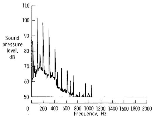
Fig. 4 Narrowband analysis at microphone 2 for the flight conditions of run 1 (treated airplane).
