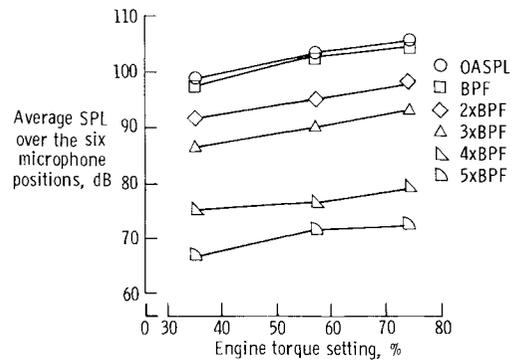
**Fig. 10** Effects of engine torque on space averaged sound pressure levels for the treated airplane.
