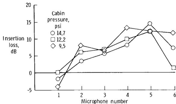
Fig. 6 Spatial variation of the insertion loss at  $2 \times \text{BPF}$  (210 Hz) for three cabin pressures.
