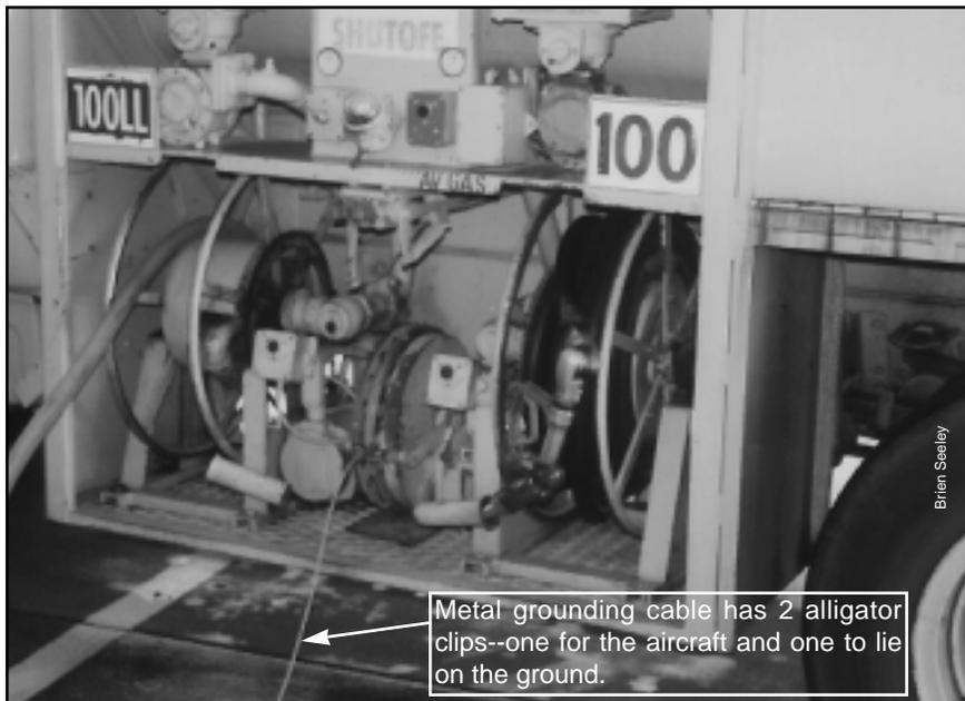
equipped with fiberglass fuel tank(s), the fuel tank filler neck(s) may not be grounded. Homebuilders of such aircraft should make a special point of attaching an internal grounding wire from the tank filler neck to the aircraft's metal ground bus, and this, in turn, should be grounded to the landing gear.
