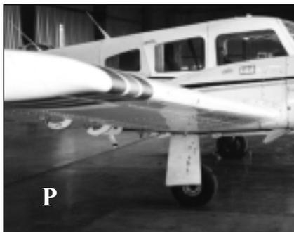
One variation of this is leading edge droop. (P). This produces a local increase in the lift coefficient and is a part of many STOL kits for production aircraft. It typically improves the ability of its local portion of the wing to keep flying when other, non-drooped portions of the wing have stalled. The drooped portion is often forward of an aileron and thus helps the aileron to remain effective during a stall.
