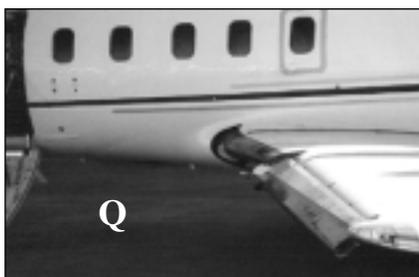
can increase a wing’s lift coefficient by up to 40%. Unlike trailing edge flaps, which allow the tilting of the fuselage nose-down for better visibility during approach, leading edge slats do
