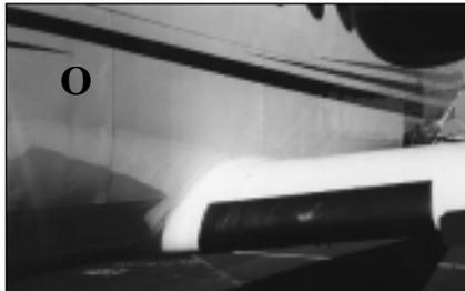
tion of lift and the stall progression along the span to be tailored without the use of wing twist. It may also reduce airflow separation at the fuselage/wing root junction.
