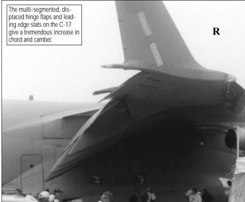
The multi-segmented, displaced hinge flaps and leading edge slats on the C-17 give a tremendous increase in chord and camber.
