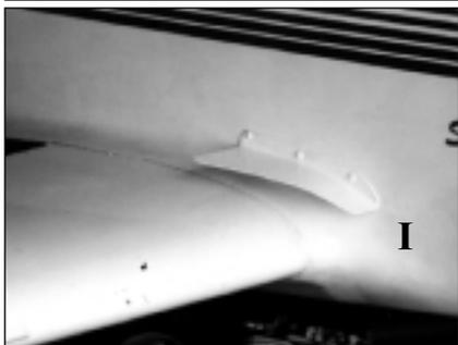
provide lift, increase local effective sweep angle and enhance pitch and yaw stability as well as to cleanly house a tailwheel assembly or tail skid. (A).
