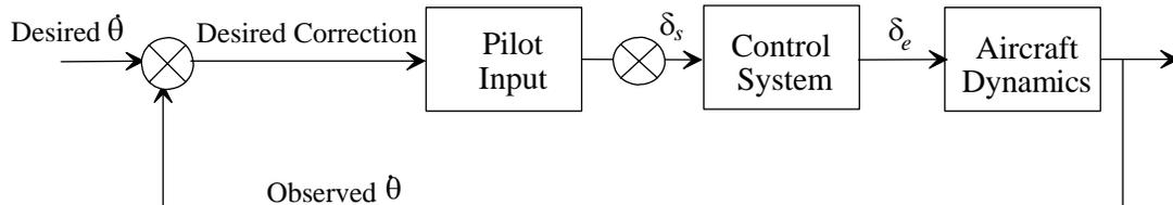
Figure 13.2 Aircraft Closed Loop Block Diagram
