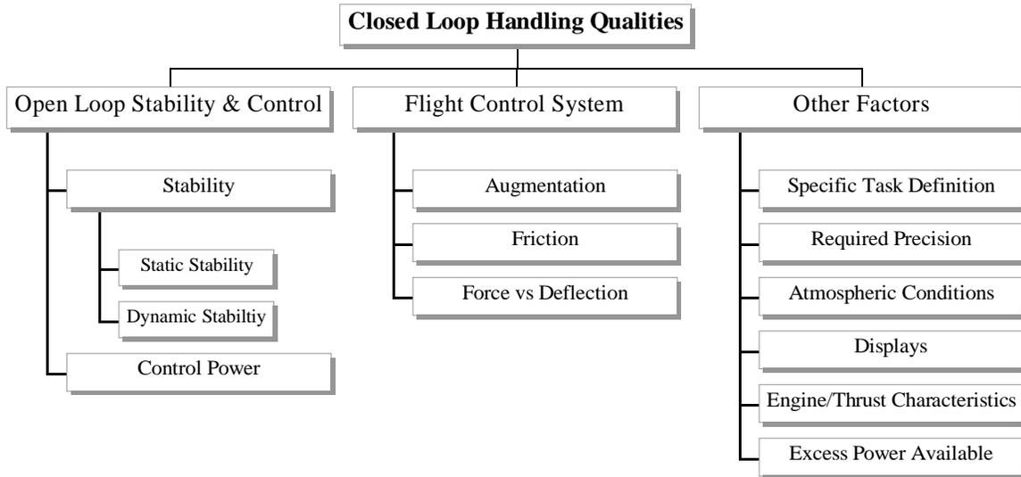
Figure 13.1 Elements of Closed Loop Handling Qualities
