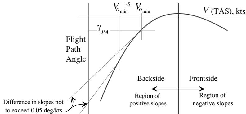
Figure 13.7 Aircraft Performance Specification Flight Path Stability
