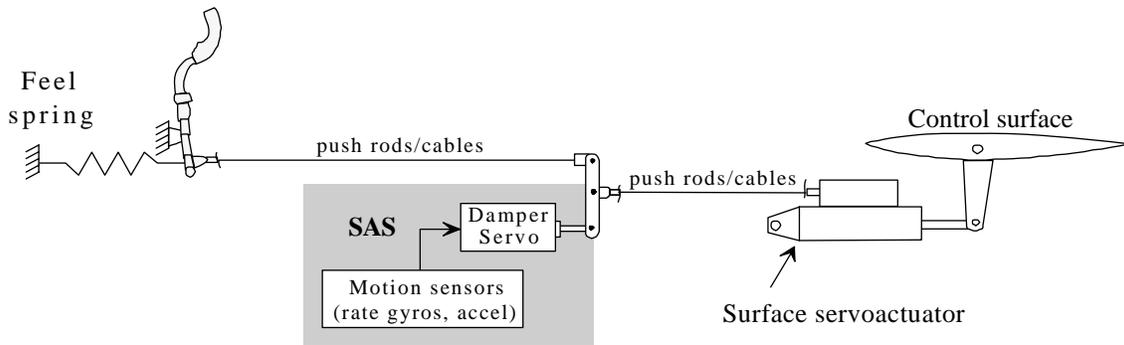
Figure 13.9 Stability Augmentation System
