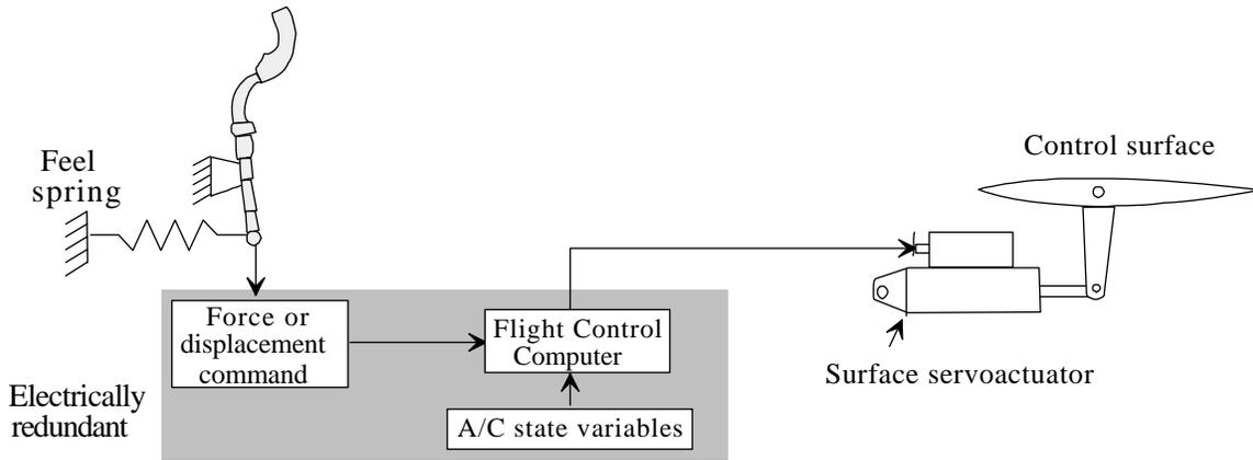
Figure 13.12 Fly By Wire Flight Control System
