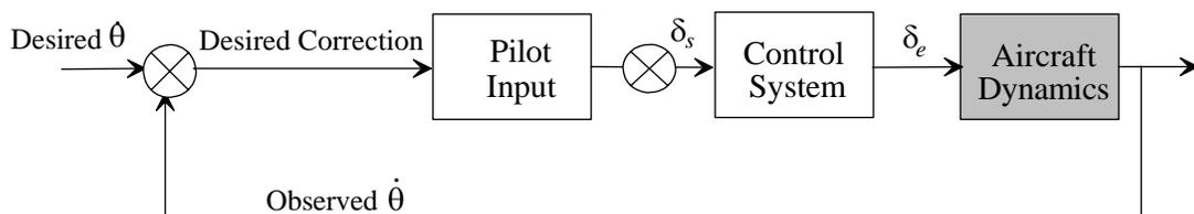
Figure 13.5 Aircraft Dynamics in the Closed Loop
