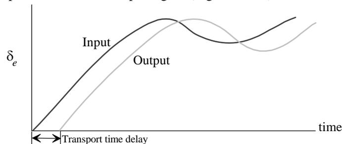
Figure 13.14 Transport Time Delay
