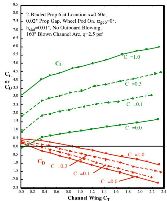
Fig. 6– GTRI Test Results: Prop Thrust Effects on Lift and Drag at Constant Blowing and  $\alpha=0^\circ$
