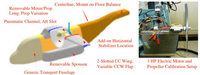
Half-span Powered Pneumatic Channel Wing Model with 3 Air Blowing Slots per wing (1 in Channel, 2 in CCW)
