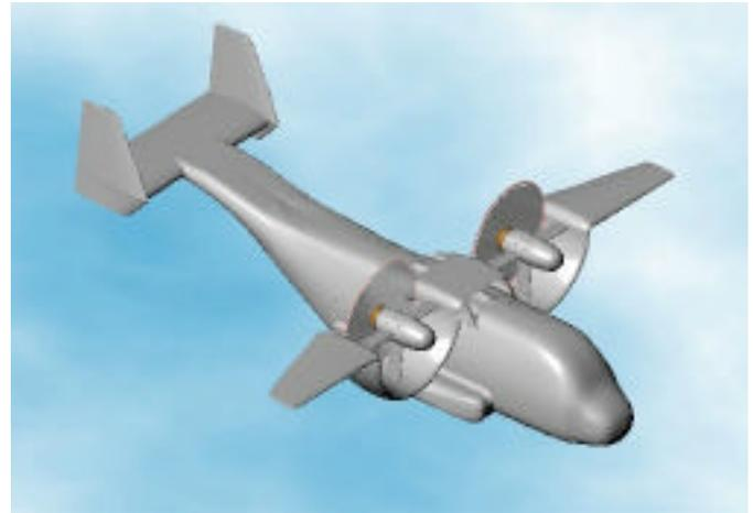
Fig. 3 – Conceptual Pneumatic Channel Wing Super STOL Transport Configuration
