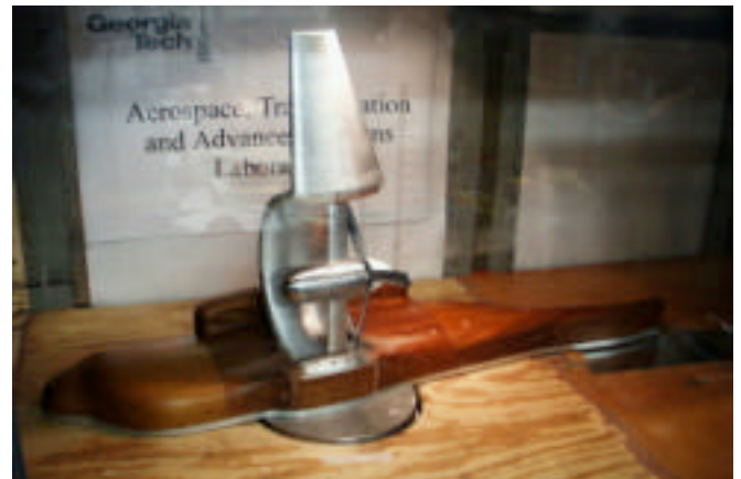
Fig. 4 – Pneumatic Channel Wing/CCW Semi-span Model Design, Power Unit, and Installation in GTRI Model Test Facility Research Tunnel (Outboard CCW Unblown Here)
