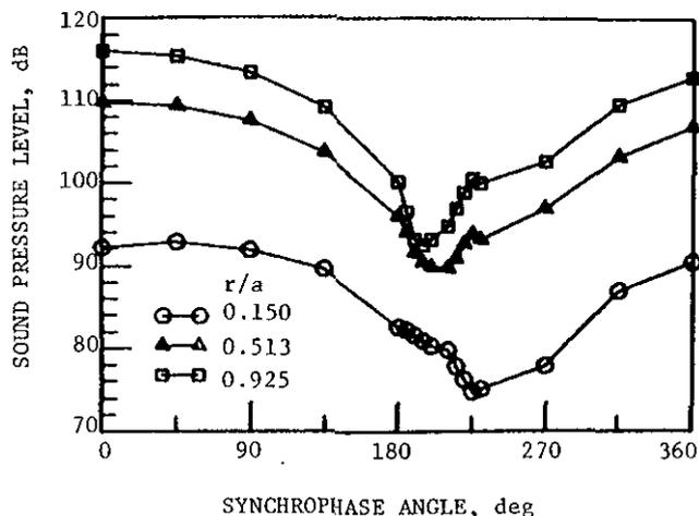
Fig. 6 Interior Pressure Measurements at  $x/a = 0.0$ ,  $\theta = 0^\circ$  and  $f = 680$  Hz.
