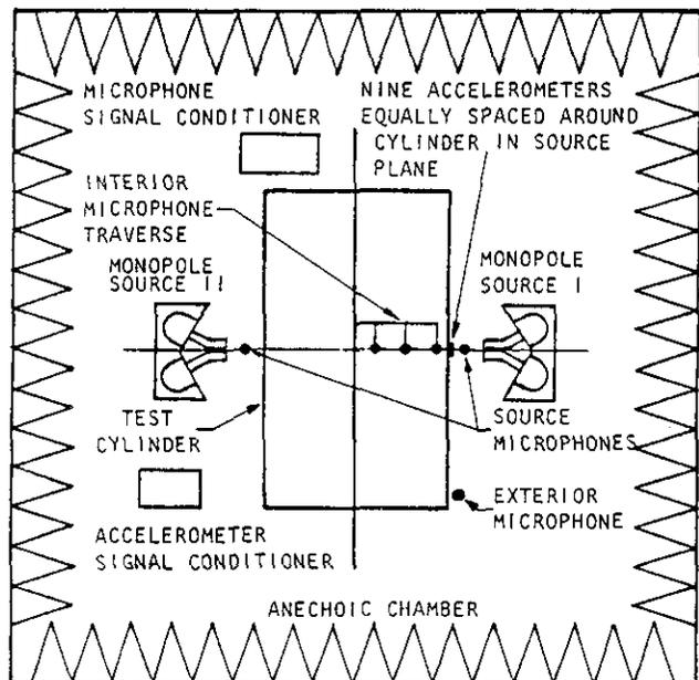
Fig. 2 Schematic Diagram of Experimental Setup.
