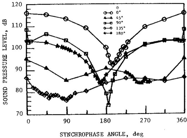
Fig. 9 Interior Pressure Measurements at  $x/a = 0.0$ ,  $r/a = 0.925$  and  $f = 680$  Hz.
