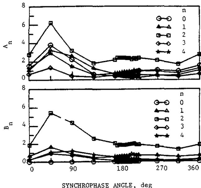
Fig. 5 Relative Modal Amplitudes of the Cylinder at  $x/a = 0.0$  and  $f = 680$  Hz.
