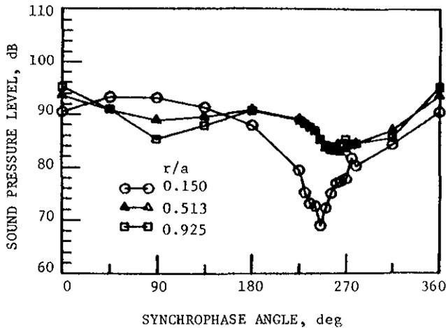
Fig. 7 Interior Pressure Measurements at  $x/a = 0.0$ ,  $\theta = 45^\circ$  and  $f = 680$  Hz.
