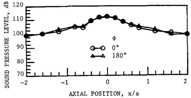
(a) Axial Pressure Distribution at  $\theta = 0^\circ$
