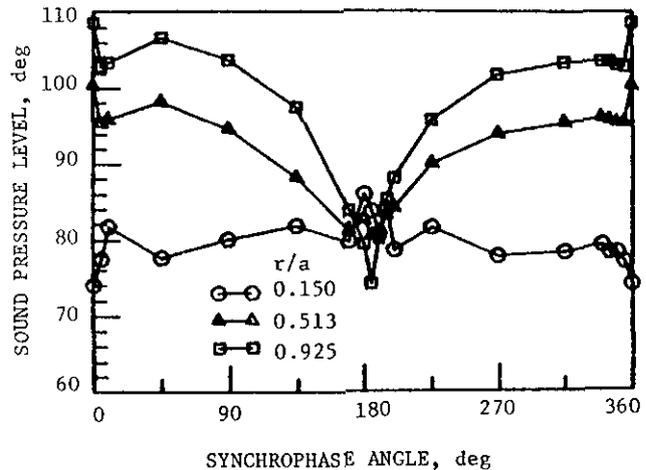
Fig. 8 Interior Pressure Measurements at  $x/a = 0.0$ ,  $\theta = 90^\circ$  and  $f = 680$  Hz.
