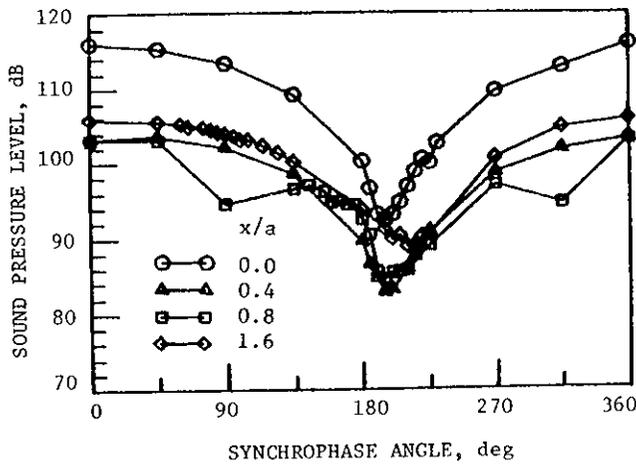
Fig. 10 Interior Pressure Measurements at  $\theta = 0^\circ$ ,  $r/a = 0.925$  and  $f = 680$  Hz.
