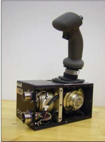
NASA's Naturalistic Flight Deck uses this fly-by-wire side-stick control with Stirling Dynamics servo motors and built-in strain gauge sensors.
