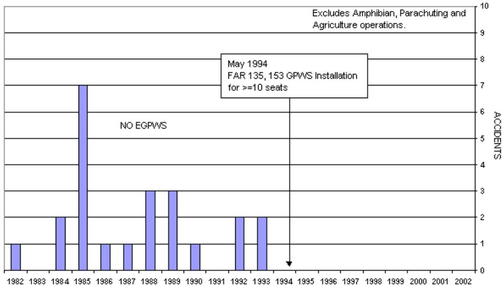
Figure 6: Effect of GPWS on CFIT accidents
